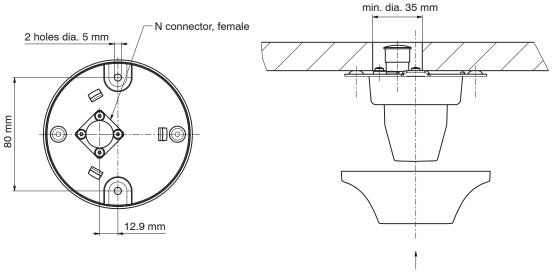
Clip the protective housing into position after the antenna has been mounted with the help of the three supplied screws.
